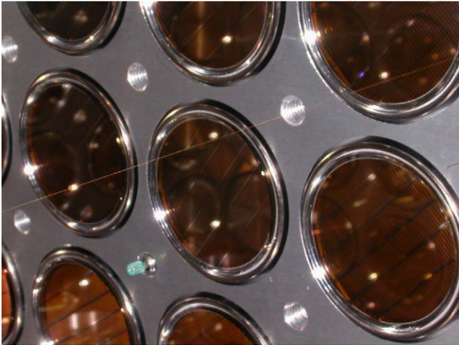
Fig. 2. A two-source wire mounted in the Calorimeter Prototype detector.
