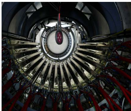
Fig. 3. Drift chambers and muon stopping target installed inside the COBRA magnet.
