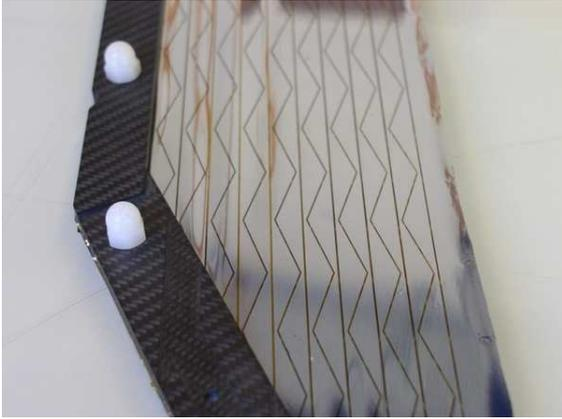
Figure 3: Double wedge or vernier pattern structure etched in the aluminum layer of the cathode foil.
