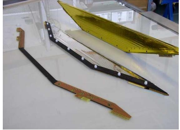
Figure 2: Anode frame with wires (front), "middle cathode" and "hood cathode" (back) of a drift chamber module.
