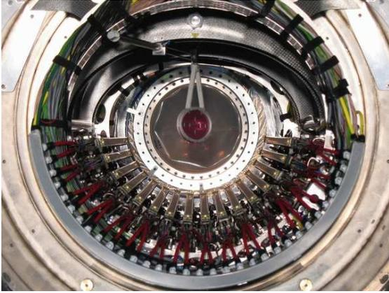
Figure 1: View of the drift chamber system from the downstream side of the MEG detector. The drift chamber modules are mounted in a half circle, whereas the muon stopping target is placed in the centre.
