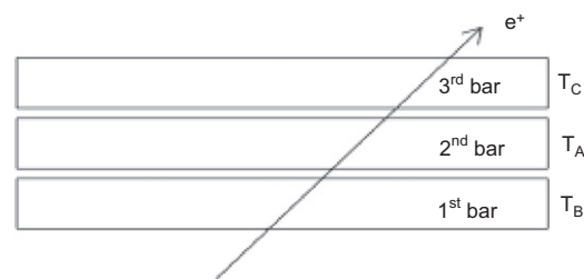
Fig. 6. A positron crossing three adjacent bars, each providing a time measurement T_X .
