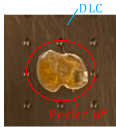
Fig. 9. DLC peeling. The orange area in the center has DLC peeling off, exposing the base material polyimide.
