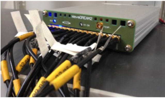
Fig. 1. WaveDREAM board in standalone configuration, used during detector commissioning and signal checks.
